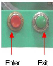
After opening the machine door, you will find there are two buttons on the right of the control board, one is red and the other is green. In this menu all the functions are almost finished by pressing two buttons. (Refer to the left picture)
